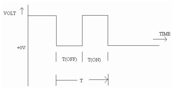
The motor will rotate during the ON time and will remain ideal during OFF time. By varying the pulse width of rectangular waveform we can vary the speed of DC motor. The direction of motor can only be change by changing the polarity of applied voltage.
